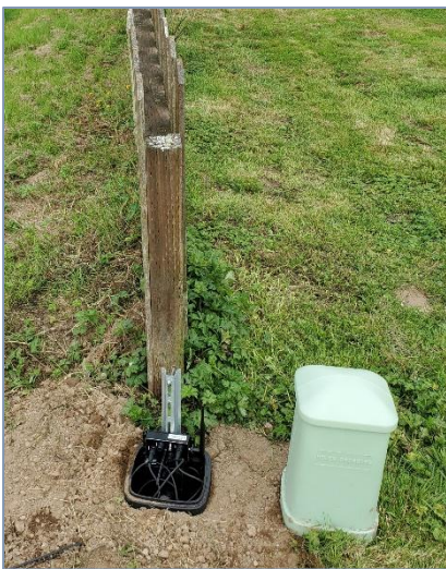
Example of a pedestal that has been used in the past to house monitoring equipment where there was no dedicated air terminal or existing pedestal. (not solar compatible).
